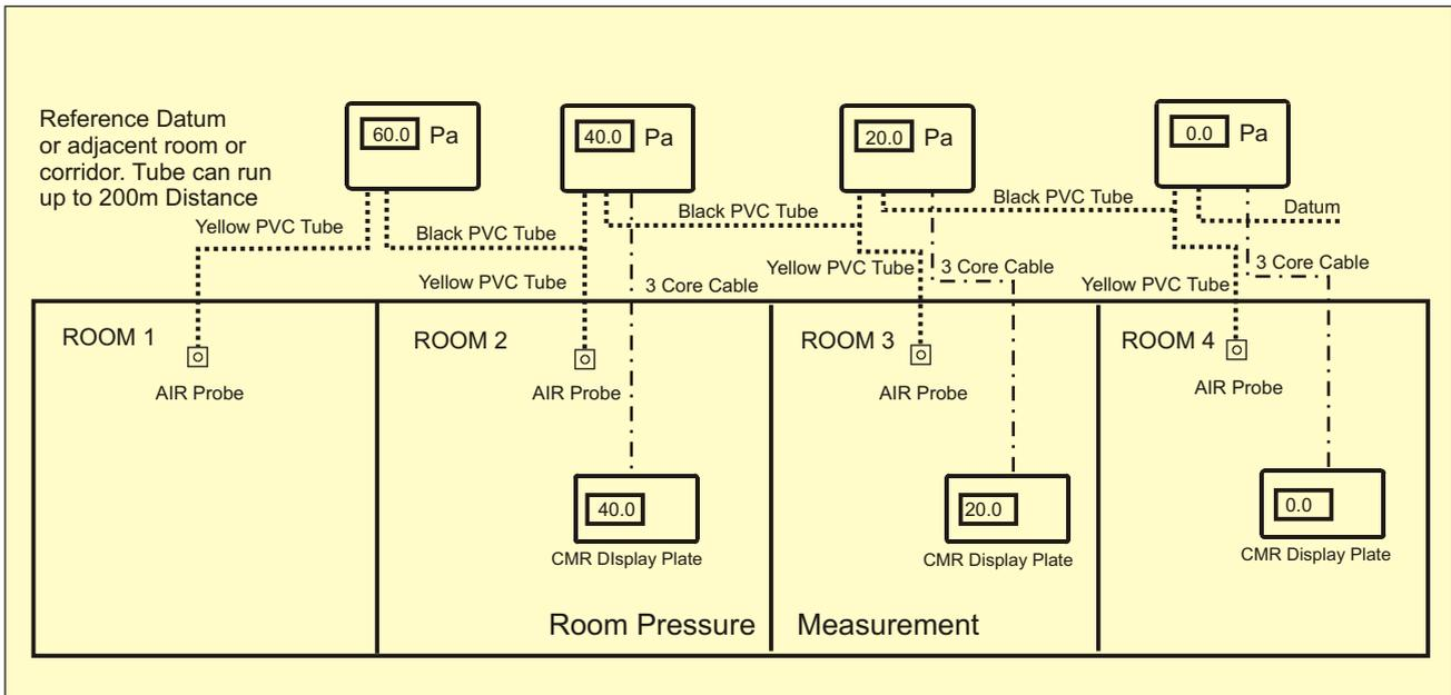
The above schematic shows a typical clean room. The room pressure must be measured against the adjacent room. Each room has air probe plates fitted to the ceiling. The air probes are connected to the P-Sensors with colour coded CMR PVC Tubing.
