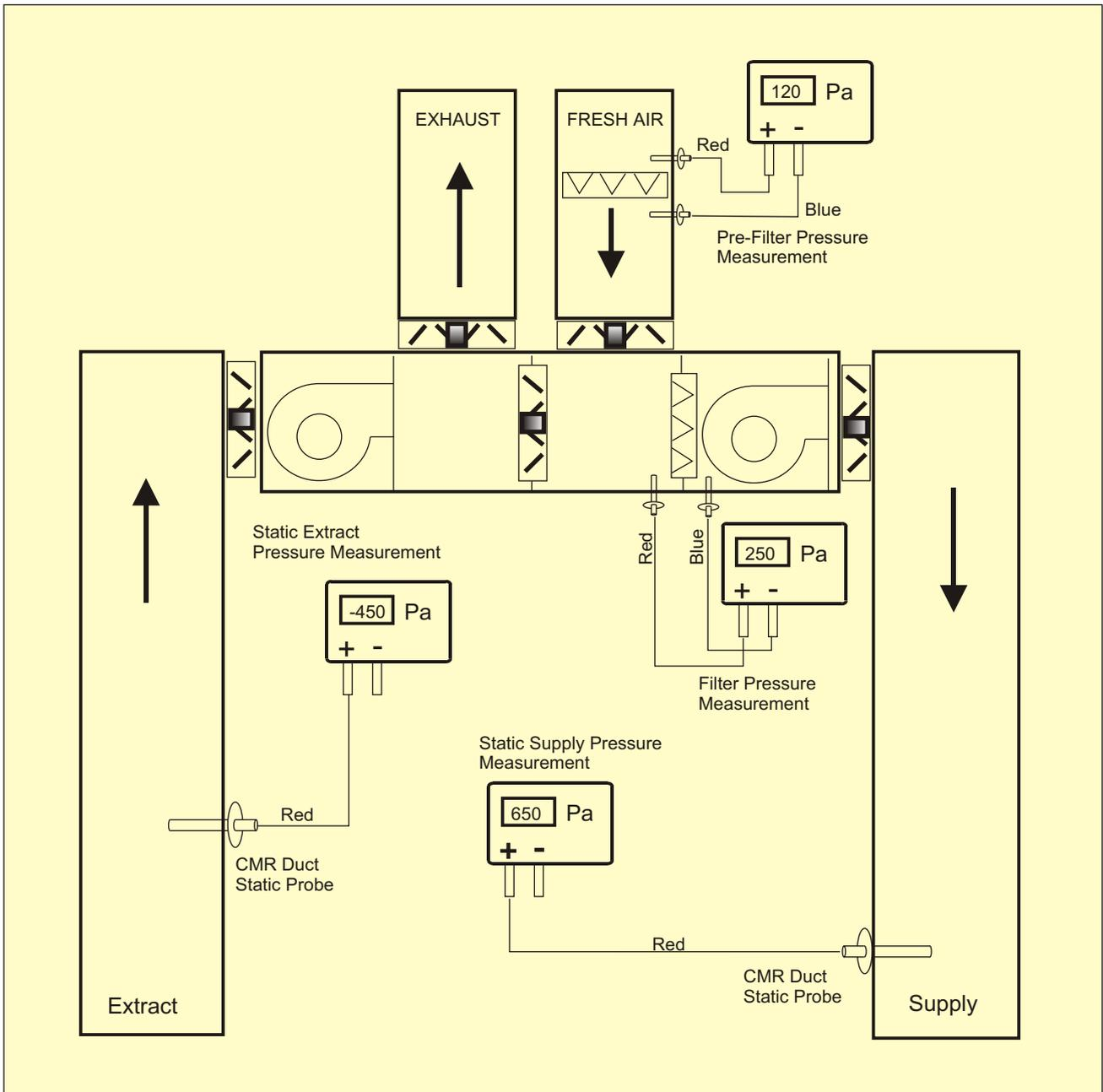
The above schematic shows a practical application in Supply and Extract Air-Handling Unit Control Systems, where Supply and
