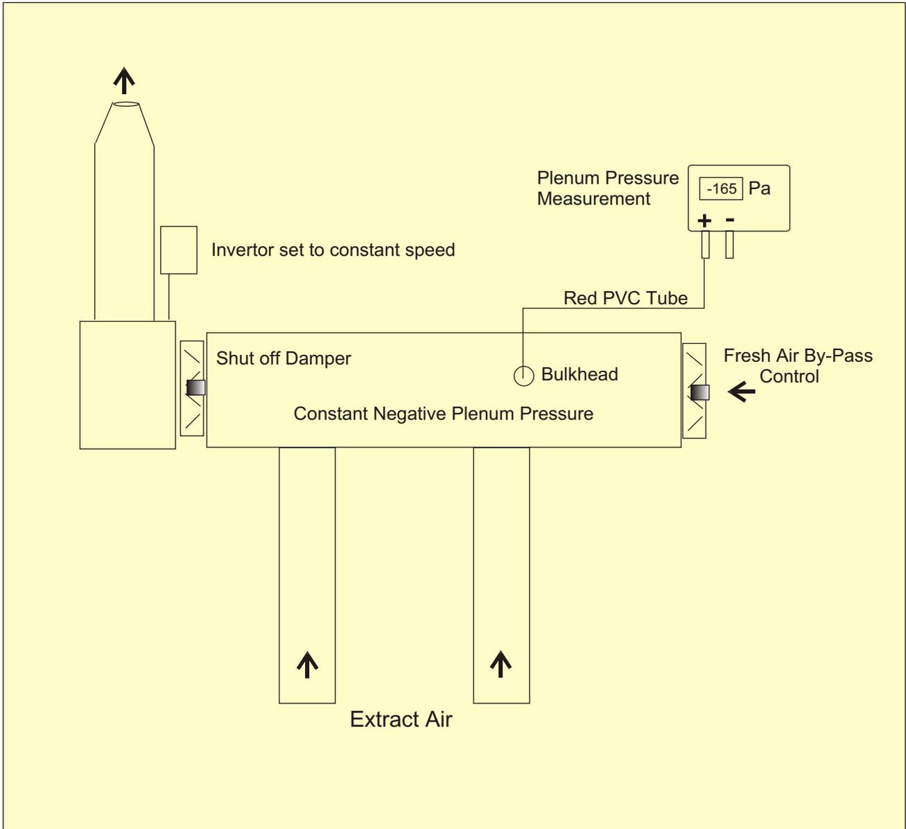
The above schematic shows a practical application in Fume Cupboard or Dust Extract Control Systems, where Plenum Pressures have to be kept constant at any time.
